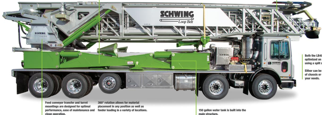
High-strength tubular steel welded boom structure and feed convevor are stronger and lighter weight than competitive aluminum booms.
